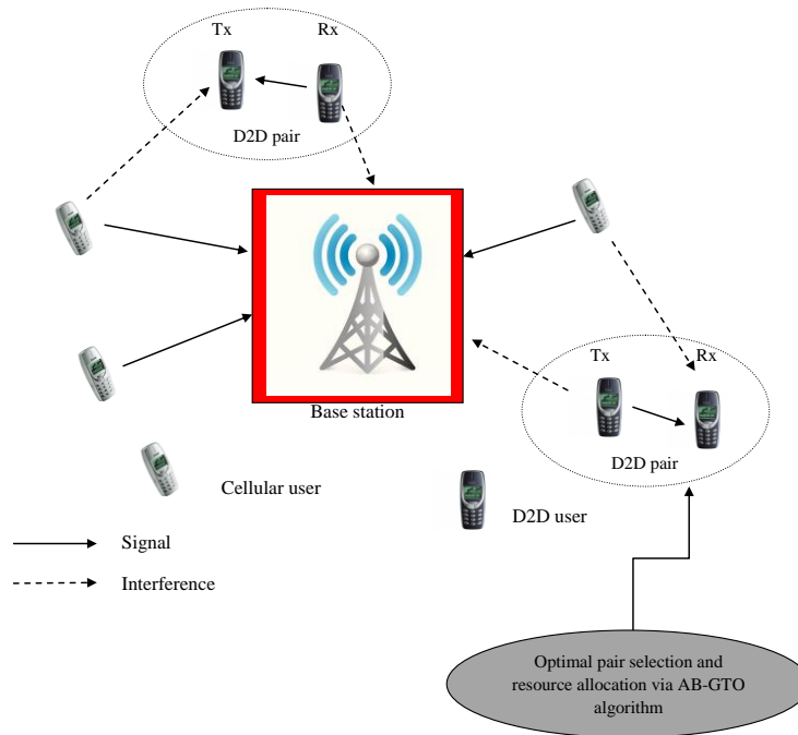
Figure. 1 Architecture of proposed REFD2DC in LTE-A system
