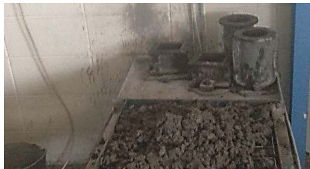
Fig.5- Casting of concrete specimens
