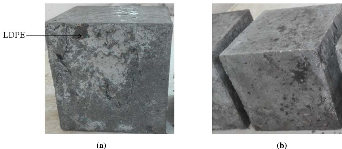
Fig. 10- views of specimens after compression test (a) CP10 and (b) CP5
