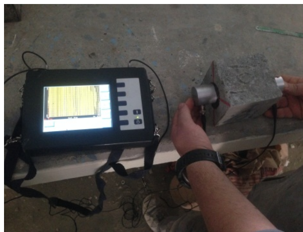
Fig. 7- UPV test of cube specimen
