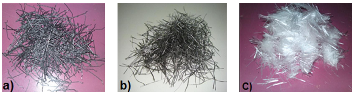
Fig. 12 - Different fibres used in pervious concrete.
