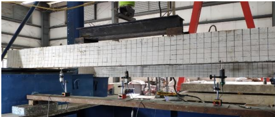
Fig. 20–Experimental test setup of RC beams
