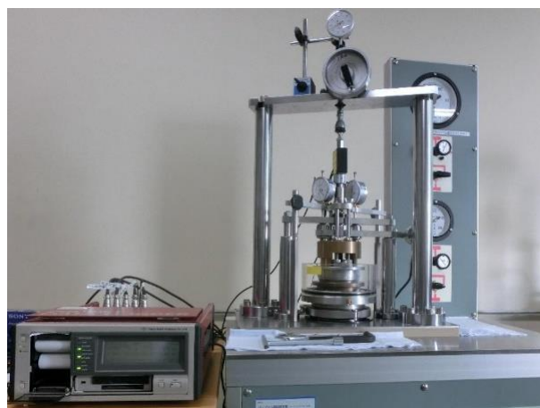
Fig. 1 –Ring shear apparatus (Bishop's type) [9, 11]
