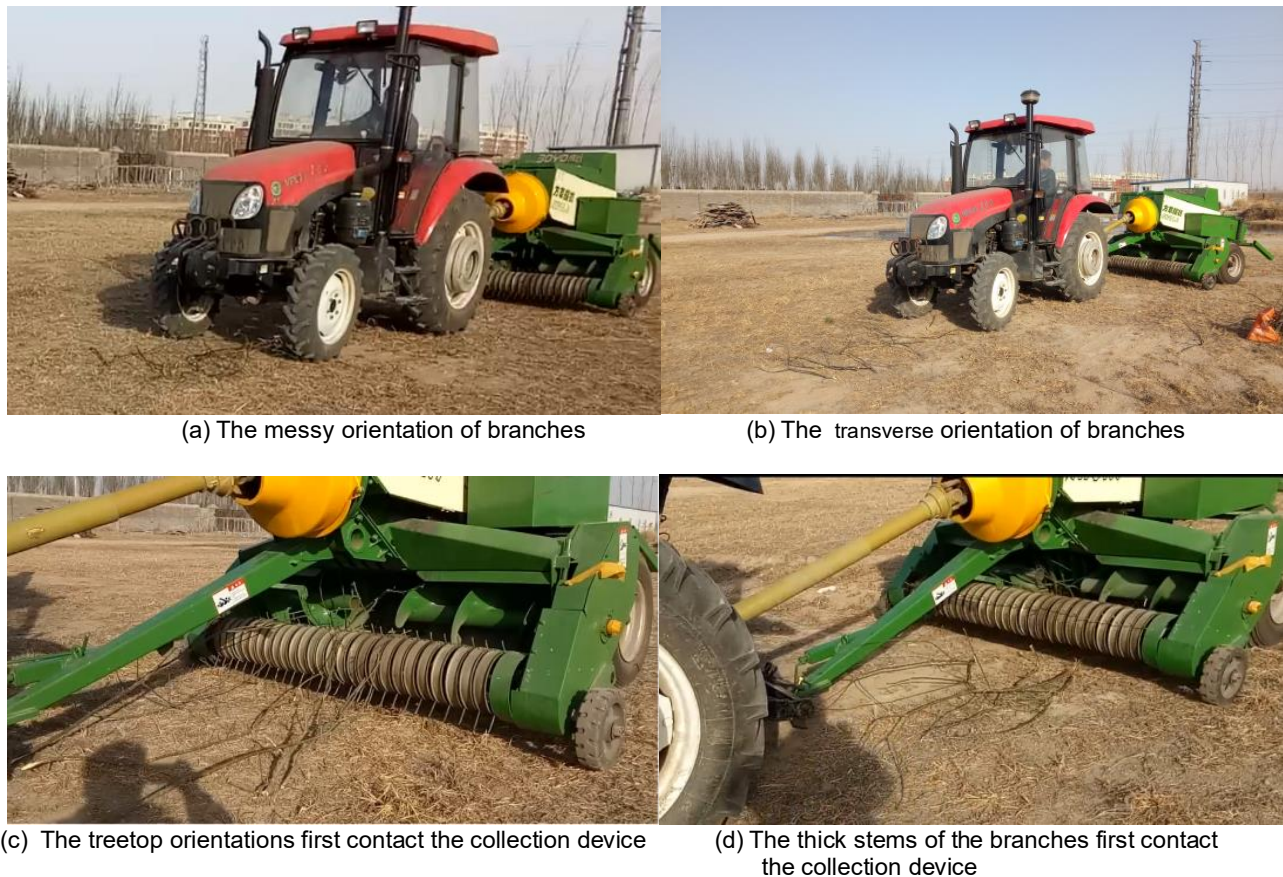
Fig. 6 - The influence of different orientations of branches on the success rate of picking
