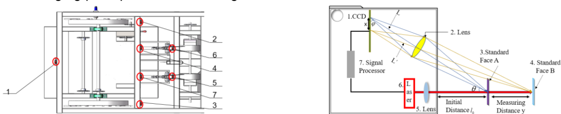
Fig. 3 - Ranging principle diagram of laser triangular reflective displacement sensor
