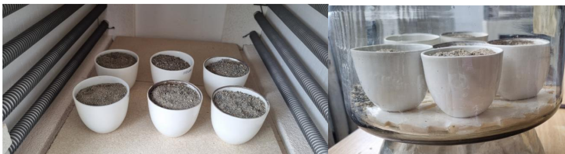
Fig. 3 – Soil samples in the oven and exicator
