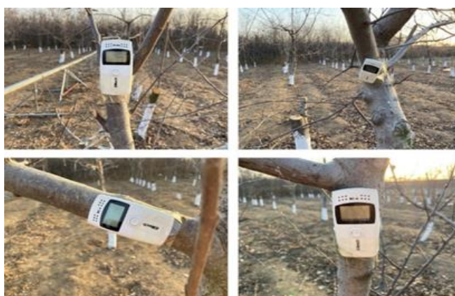
Fig. 10 - Installation of RC-4 temperature recorder
