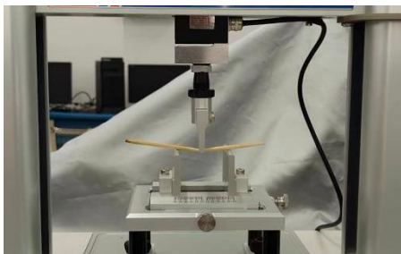
Fig. 1 - Three-point bending physical test
