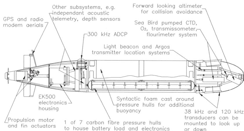
**Fig. 11 - View of Autosub-2 with the payload configured for acoustic surveys of aquatic fauna - SIMRAD EK500, scientific, multi-frequency vertical echosounder (Fernandes et al., 2003)**
