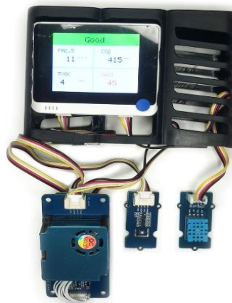
Figure. 2 AIoT electronic nose module
