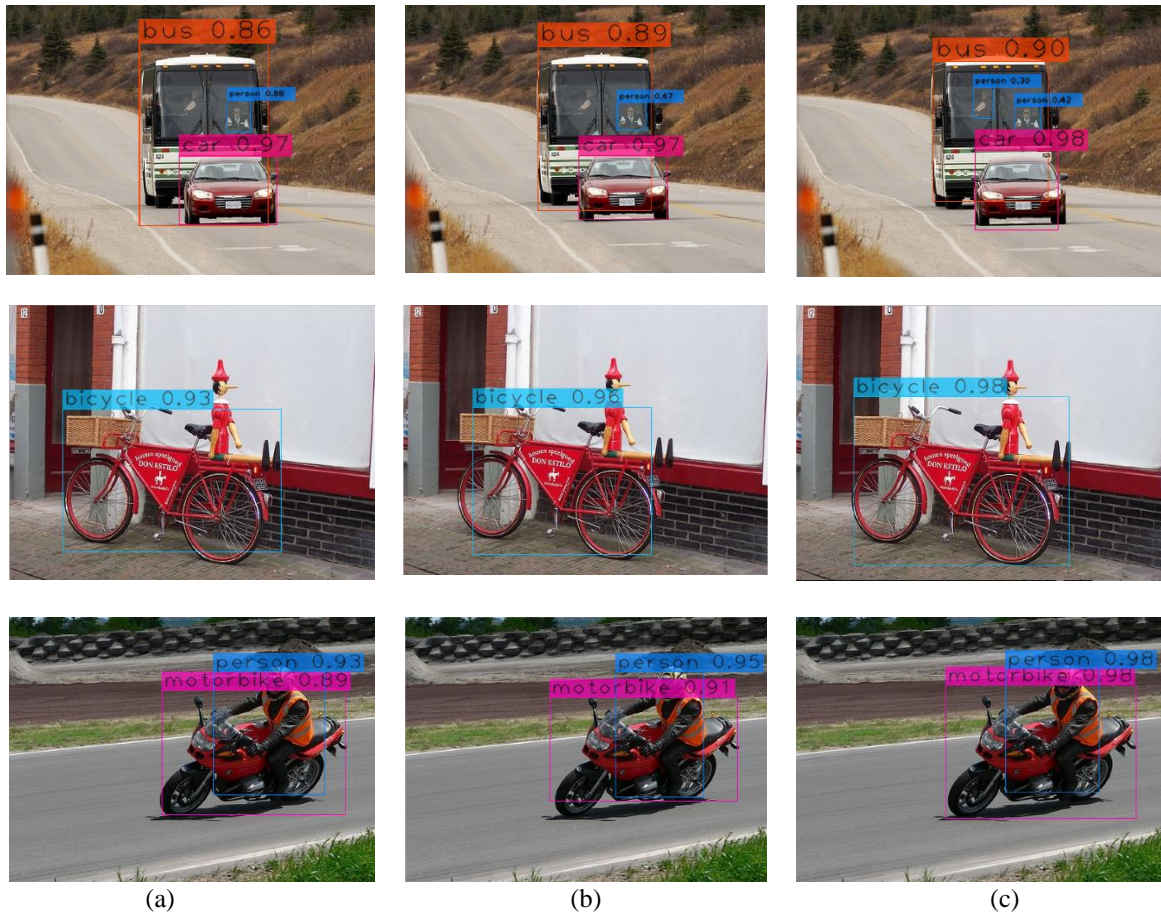
Figure. 9 Example results from PASCAL VOC 2007 dataset trained using: (a) GIoU loss, (b) CIoU loss, and (c) Proposed GCIOU loss
